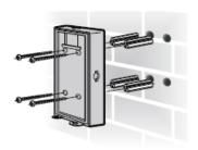
3.slip the PIR Solar Spotlight body up to down until the hasp inside is connected, fixthe body with screws.
